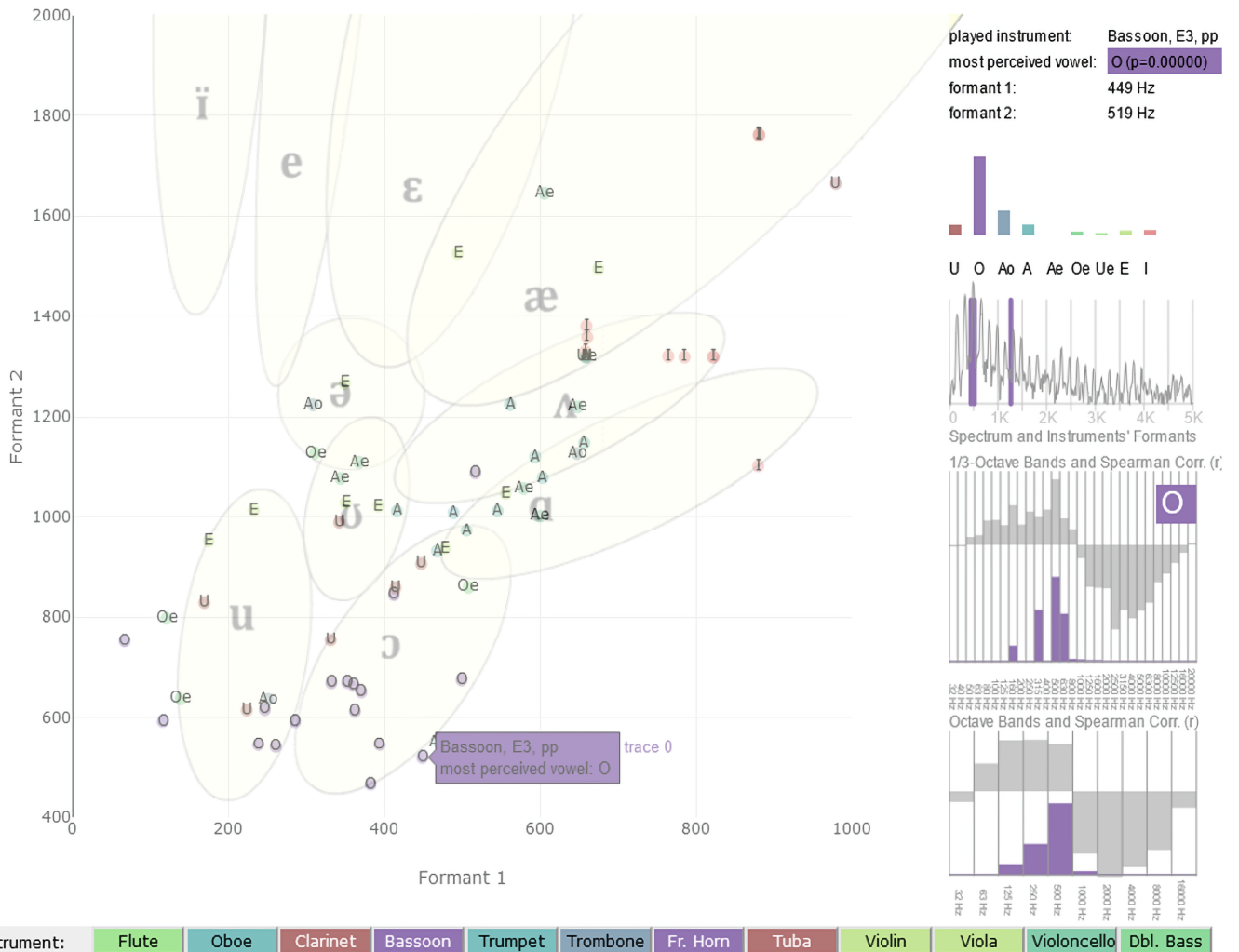
Figure 5: Interactive visualization of the vowel similarities of the instrument sounds in a vowel trapezoid (Formant 1 and 2 on the X and Y axes) combined with — on the right side — a display of the strength of the selected vowels, the formant ranges detected in the spectrum as well as their third octave and octave band spectra.
